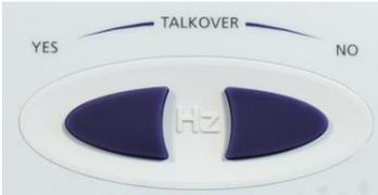
To use the counter the operator selects the frequency buttons: left for **YES** or right for **NO** according to the response made by the patient.
