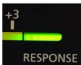
When the test person is pressing the patient response switch, the LED above the display labeled with **RESPONSE** will illuminate.
