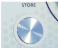
The store button is located to the left of the Channel 2 rotary control (attenuator). The button is conductive, by touching it the current test level and frequency will be stored to the temporary memory of the device.
