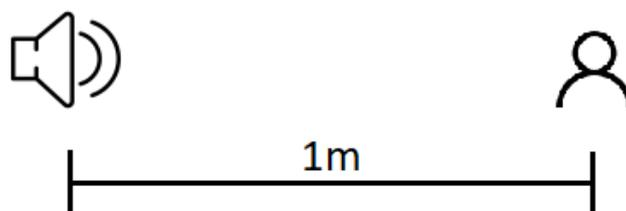
For calibration, the measuring microphone of a sound level meter (SLM) is placed at the reference point (the point that the subject's head will be located).
