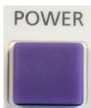
Select the POWER button for 1 second to switch the instrument on. The display will briefly show the model and the type of headphone currently selected for use. No warm-up time is required, although a short diagnostic routine will run for a few seconds.
