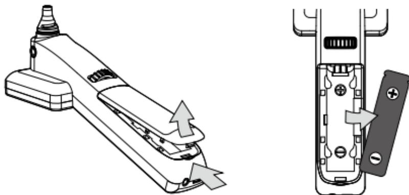
Open the battery cover by digging out the gap in the bottom of battery cover with a finger or something pointed.
