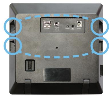
Your Ensemble is nearly ready to use right out of the box. The stand snaps into two slots on the back of the phone. Use the two lower slots to hold the phone more upright; the upper slots hold it a little more horizontal. Next, remove the two clear protective covers. The power cord and the telephone cord on the back of the phone unwind by pulling gently. Plug the power cord into any wall socket or extension cord and you're ready to proceed.
