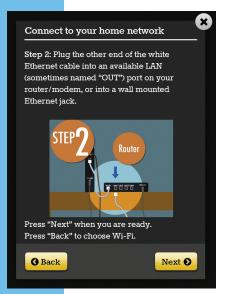
Next is connecting to the Internet. Your Ensemble will connect to your modem or router either with an Ethernet cable, which is provided in the box (the white cable) or wirelessly (using Wi-Fi). If you're using Ethernet, there's a short video to show you where to plug in the white cable.
