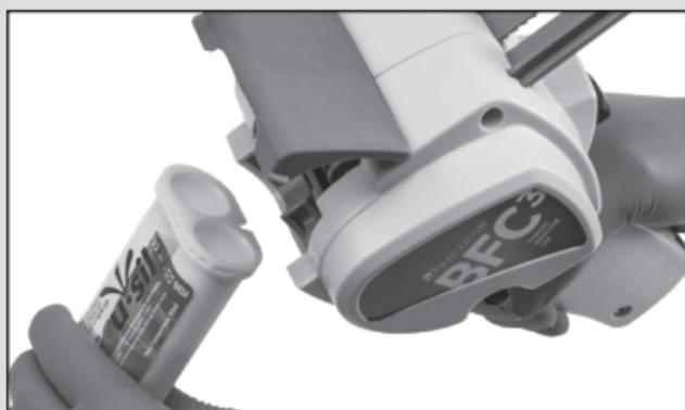
Insert material cartridge into BFC<sup>3</sup> with the cartridge notch facing down. Close the cartridge door completely.
